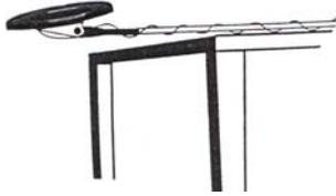
5. Slowly sweep a sample of the material you want the detector to find (such as a gold ring or a coin) 2-3 inches or more above the face of the search coil. When the detector detects any metal, it sounds a tone and an arrow appears below the target icon. Also the LCD displays the depth of the target.
